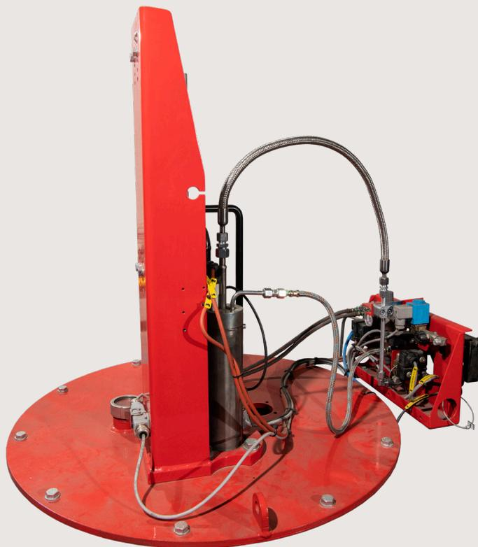
The flexible fuel oil hose modification kit contains everything needed for vertical mounting of the flexible fuel oil hose on your Alfa Laval Aalborg KBSD/A burner. Mounting in a vertical position will decrease the tension placed on the hose when the lance is in movement.
