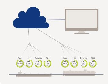
Benchmarking – PureSOx Connect benchmarking features make it possible to compare the connected vessels within your fleet. They assist you in benchmarking each vessel's PureSOx performance to reach higher levels of optimization, which reduces your operating costs over time.
