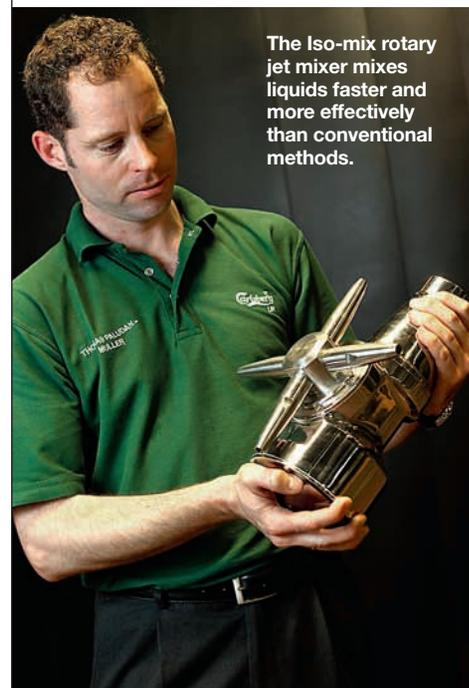
The Iso-mix rotary jet mixer mixes liquids faster and more effectively than conventional methods.
