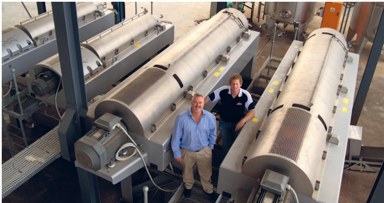
The three-in-one Foodec decanters replace traditional separation, pressing and settling, reducing process time by 24 hours.
