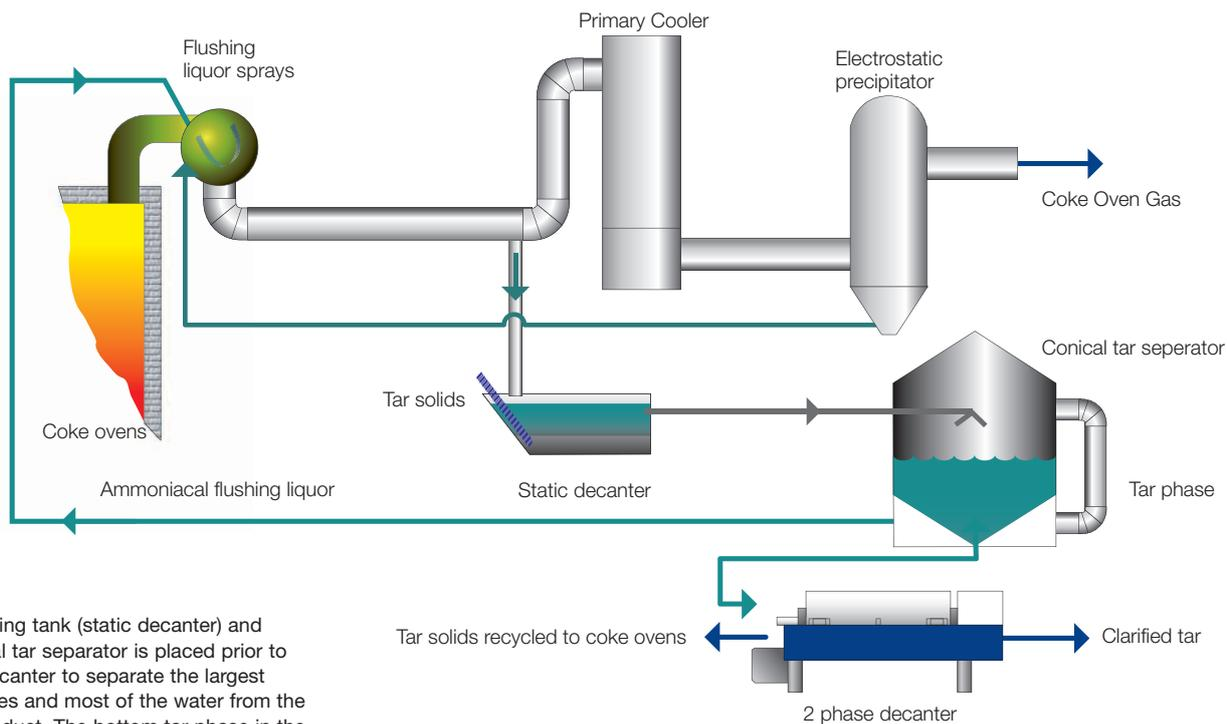
A settling tank (static decanter) and conical tar separator is placed prior to the decanter to separate the largest particles and most of the water from the tar product. The bottom tar phase in the conical tar separator is then pumped to the decanter for further clarification.
