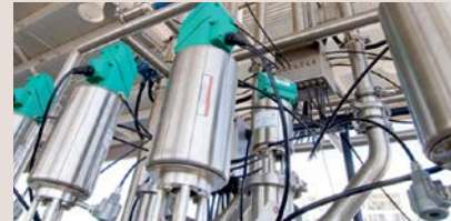
Alfa Laval Tri-Clover 700 series valves Tri-Clover 700 series provide years of reliable performance. Rugged plastic stem bushings eliminate metal-to-metal galling. The stem is threaded to the actuator shaft, eliminating the coupling between the stem and actuator, thereby ensuring proper alignment. Bushings at each end of the cylinder support stem also ensure perfect alignment. Each valve features a heavy-duty bonnet and body ferrule design that will stand up to years of pounding from hydraulic shock.
