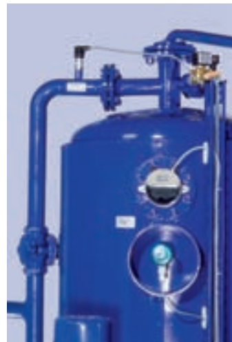
Fig. 4 External side glass and foam detection on the vacuum tank
